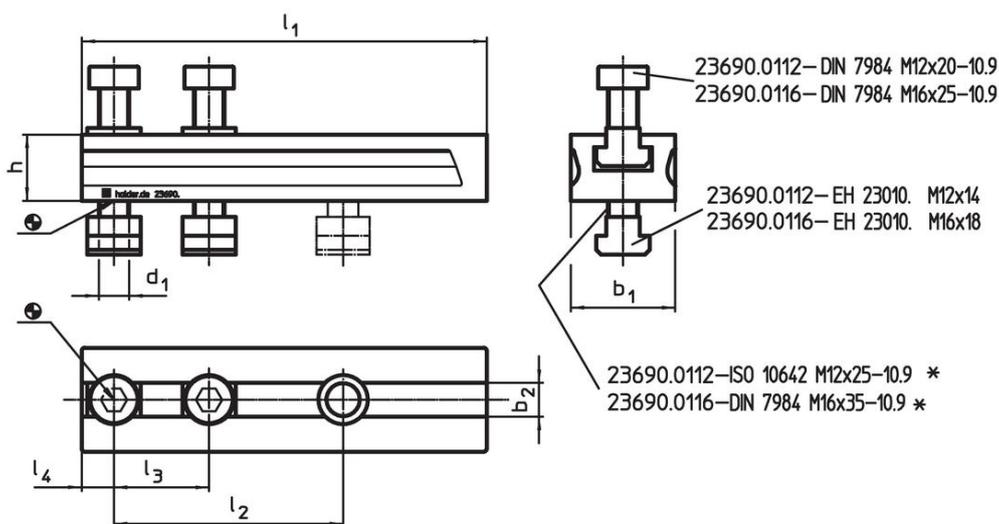
\* When using more height adapters the screws ISO 10642 or DIN 7984 have to be replaced by screws extended by the dimension h.
